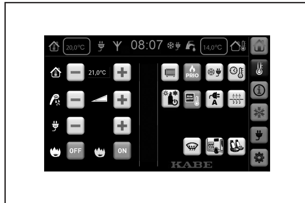
The motorhome control panel's Heating menu.
