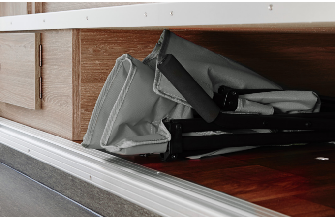
In KABE's fully integrated models, the space between the double floors is utilised in a smart way*. In Travel Master i810 LQB, you can access the storage space from the garage area.
