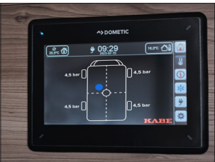
KABE Smart Level. The KABE Smart D panel includes KABE Smart Level with three useful functions. Smart Level tracks your gas level (with use of one gas bottle, not for composite bottles), tyre air pressure and the inclination of the motorhome.
