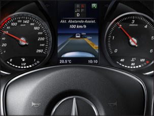
DISTRONIC adaptive cruise control. The active distance assistant DISTRONIC maintains the distance to the vehicle in front, assisting the driver on the highway or in stop-and-go traffic (standard in Imperial).
