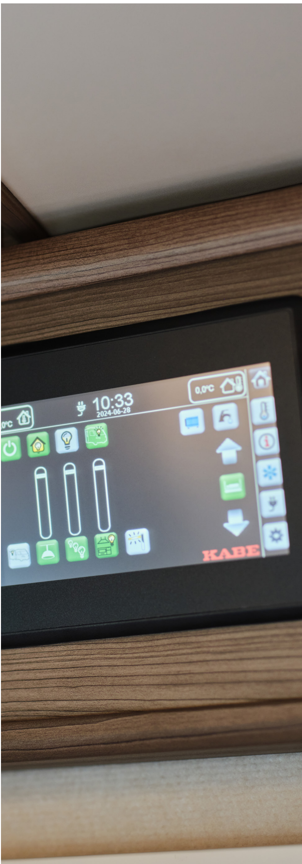
The home page shows all the controls for lighting and digital dimmer sliders. It also displays the temperature, both outside and inside, and the current time.
