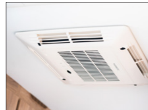
Klimaanlegg bodel Fresh Jet FJ2200 (standard Imperial)
