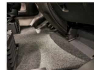
Heating carpet in cab with heated inside door step Heating exchanger
