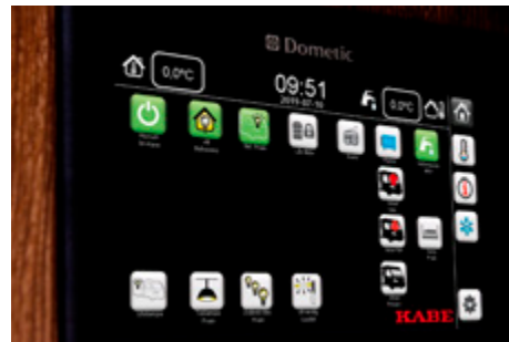
On the home page, you can see lighting controls and digital sliders for dimmers. Inside and outside temperature as well as time are also displayed.
