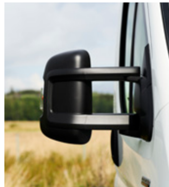
Fog-free side mirrors, electrically heated and extended.
