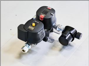
Duocontrol. Duocontrol has a built-in automatic gas switch, reduction valve and collision sensor which is triggered on impact with a G-force of 3.5 G. The supply of gas is shut off immediately to avoid a gas leak. Duo Control is approved in all of Europe and enables the gas to be on while driving.
