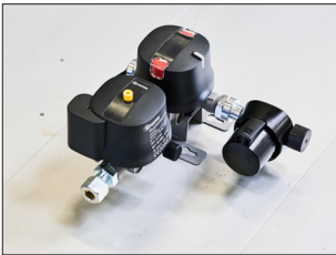
Duocontrol has a built-in automatic gas switch, reduction valve and collision sensor which is triggered on impact with a G-force of 3.5 G. The supply of gas is shut off immediately to avoid a gas leak. Duo Control is approved in all of Europe and allows for the gas to be on while driving.
