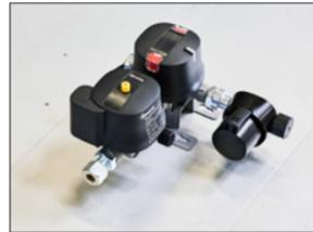
**Duocontrol.** Duocontrol has a built-in automatic gas switch, reduction valve and collision sensor which is triggered on impact with a G-force of 3.5 G. The supply of gas is shut off immediately to avoid a gas leak. Duo Control is approved in all of Europe and allows for the gas to be on while driving.
