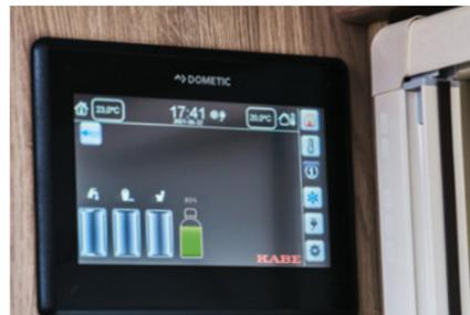
Current status information about fresh water level, waste water level and battery voltage is clearly displayed. With the new function KABE Smart Level you can also see the LPG level (for use with one LPG bottle, not for composite bottles), tire air pressure and the inclination of the caravan (standard Imperial, option for Royal).
