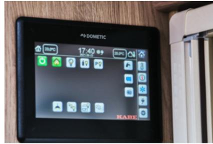
The home screen displays lighting controls and digital sliders for dimmers, inside and outside temperature as well as time.
