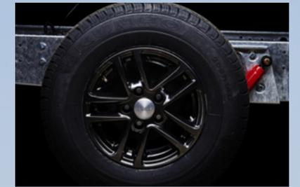
**Tyres and clutch.** Our single axle caravans feature 8-layer tyres. 14" steel rims are standard in Estate and 15" aluminium rims are available as an option with the Design Package. 15" aluminium rims are standard in Gemstone and Royal and 17" Diamond Cut aluminium rims in Imperial (available as an option in Royal). All models include friction clutch.
