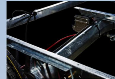
**Extra rigid chassis.** Extra beams between lengthwise chassis joists result in a more stable floor and an extra rigid chassis. Connecting beams provide the best stability possible. The chassis has outriggers from the lengthwise side beam, to relieve the weight pressure where the floor and walls are joined. The body can withstand very high loads, for example, large amounts of snow on the roof.
