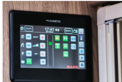
All information and controls for heating are displayed on a separate page. You can easily adjust the heat with digital sliders.
