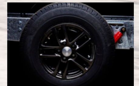
Tyres and clutch. Our single axle caravans feature 8-layer tyres. 14" steel rims are standard in Estate and 14" aluminium rims are available as an option with the Design Package. 15" aluminium rims are standard in Gemstone and Royal and 17" Diamond Cut aluminium rims in Imperial (available as an option in Royal). All models include friction clutch.
