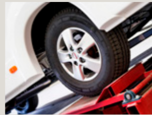
DURABILITY TEST Durability tests are performed and simulated with equipment corresponding to 10,000 km of normal driving.
