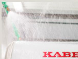
RAIN CHAMBER In the rain chamber, the caravans are tested with a high pressure sprayer.
