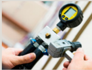
GAS The gas system is pressure tested.
