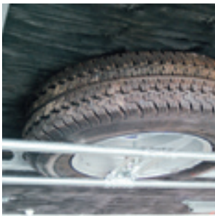
Reservehjulsholder (X0063) under chassis.
