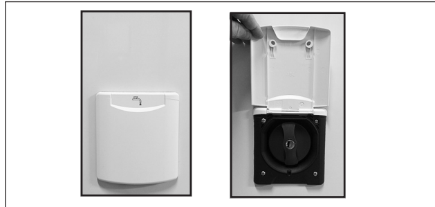
Filling with fresh water
