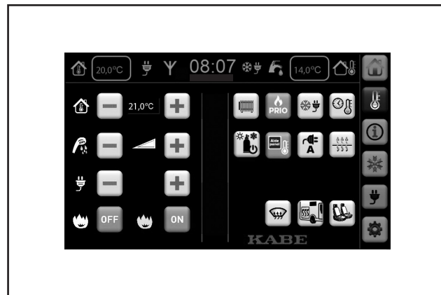
The motorhome control panel's Heating menu.
