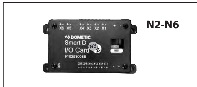
The picture shows one of the electrical system's N2 – N6 units. Dometic Smart D I/O card.
