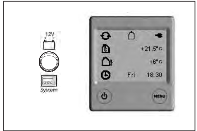
The boiler's control panel.
