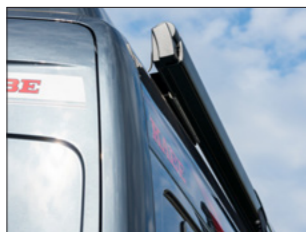
Electric awning, Thule 5200 12 V White awning 4,0 m – white van Black awning 4,0 m – blue-grey van
