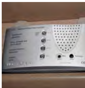
Gassalarm, sikkerhetsalarm NX5 Y0314
