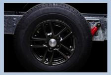
Tyres and clutch. Our single axle caravans feature 8-layer tyres. 14" steel rims are standard in Estate and 15" aluminium rims are available as an option with the Design Package. 15" aluminium rims are standard in Gemstone and Royal and 17" Diamond Cut aluminium rims in Imperial (available as an option in Royal). All models include friction clutch.
