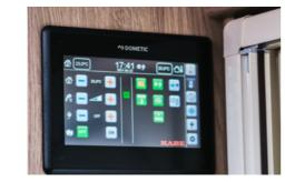
All information and controls for heating are displayed on a separate page. You can easily adjust the heat with digital sliders.
