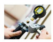
GAS The gas system is pressure tested.
