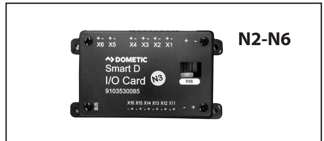
The picture shows one of the electrical system's N2 – N6 units. Dometic Smart D I/O card.
