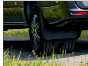
Twin wheels 4 x 2 and 4 x 4 5 ton, approx. 850 kg extra load weight, 7 ton train weight
