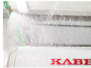
RAIN CHAMBER In the rain chamber, the motorhomes are tested with a high pressure sprayer.
