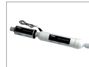
Water purification system – Alde AquaClear UV-C (Alde Compact 3030 boiler). Efficient water purification that protects the user in a gentle and eco-friendly way. Unwanted viruses and bacteria, pesticides and chemicals are removed. The water is disinfected with UV-C light generated from LEDs. In addition, the water passes through a carbon filter that removes any odour, bad taste and colour.
