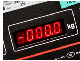
OPTIMISED WEIGHT DISTRIBUTION Scales are used to balance and optimise the weight distribution between axles.
