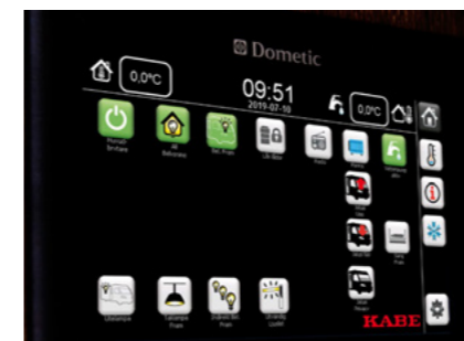
The home screen displays lighting controls and digital sliders for dimmers, inside and outside temperature as well as time.
