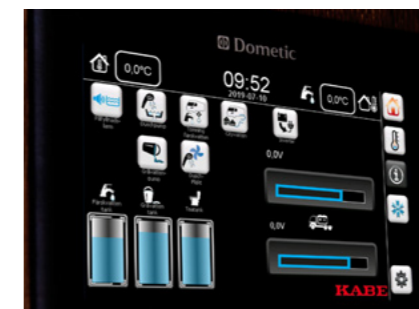
Current status information about fresh water level, waste water level and battery voltage is clearly displayed.
