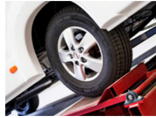
DRIVING DURABILITY TEST Durability tests are performed and simulated with equipment corresponding to 10,000 km of normal driving.
