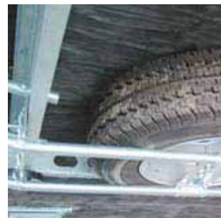
Reservehjulsholder (X0063) under chassis.
