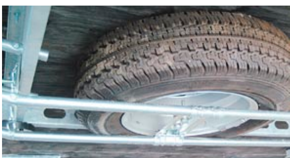
Reservhjulsholder under chassis X0063
